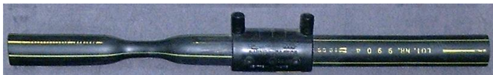
Fig. 6. Correct electro-fusion weld.
